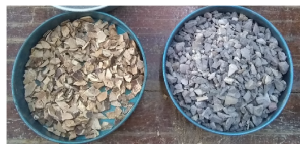
Figure 1. Appearance of CS and conventional aggregate particles (Source: Gómez-Hernández et al., 2023)
