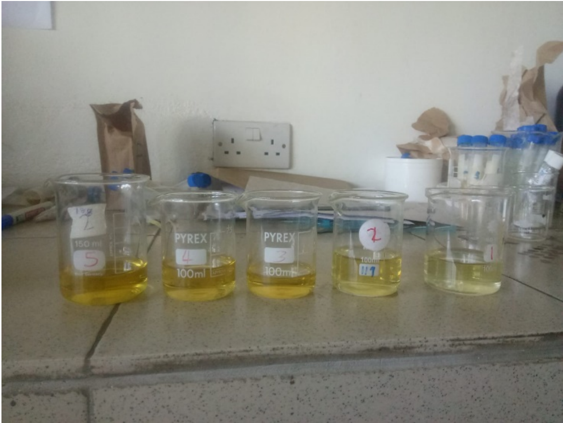
Figure 1. Appearance of the solutions of AgNPs upon reduction of 0.001 M \text{AgNO}_3 as \text{NaBH}_4 concentration decreases from 0.004 to 0.00025 M (left to right)
