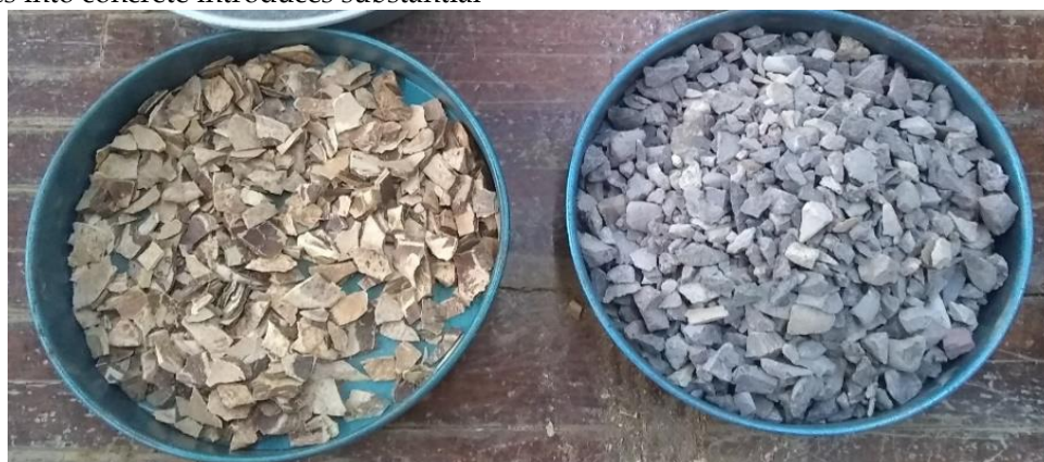
Figure 1. Appearance of CS and conventional aggregate particles (Source: Gómez-Hernández et al., 2023)
