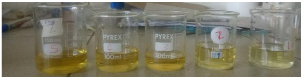
Figure 1. Appearance of the solutions of AgNPs upon reduction of 0.001 M \text{AgNO}_3 as \text{NaBH}_4 concentration decreases from 0.004 to 0.00025 M (left to right)
